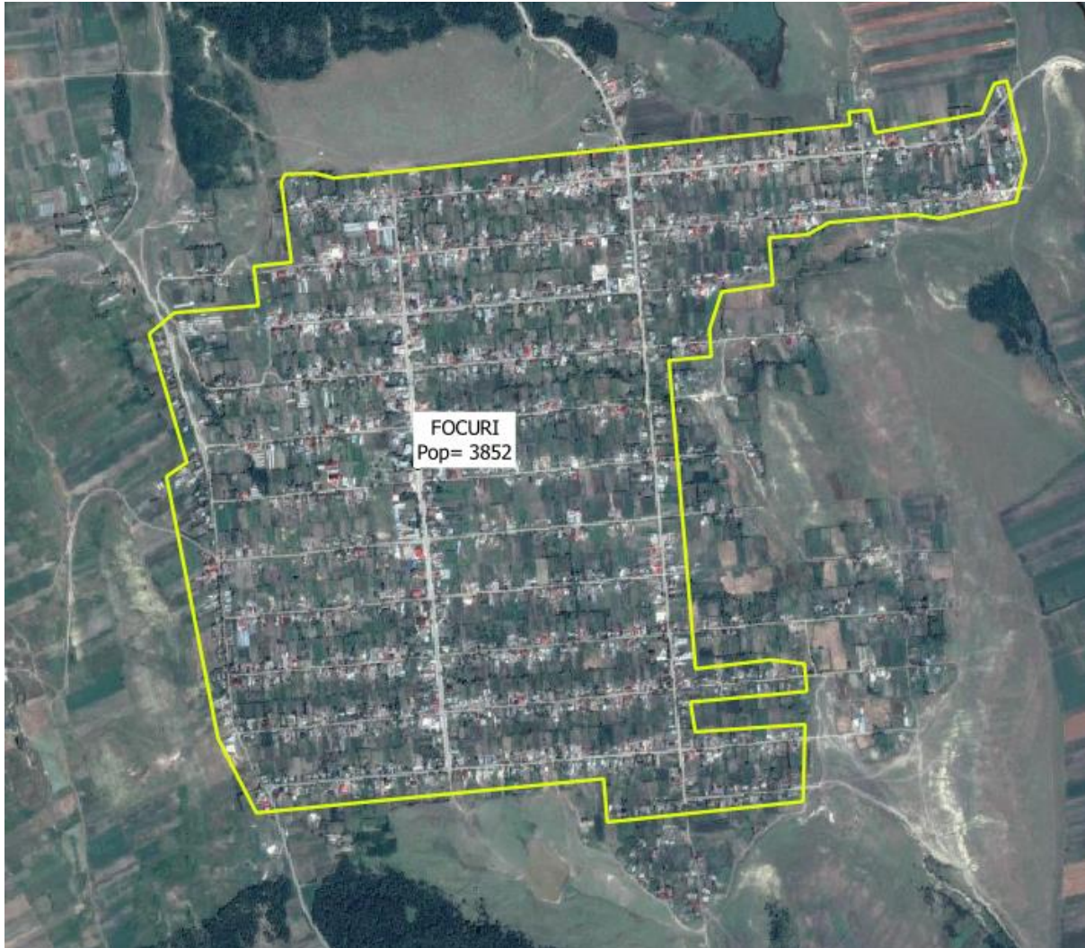
Figure 11: Visualization of included areas with high density and excluded areas with low density (where number of houses per 100 m pipe < 7)
